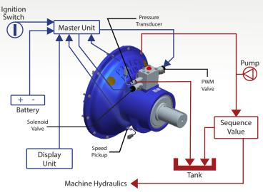
The HPTO12 is a hydraulically applied dry friction clutch for diesel engine applications. Its hydraulic design eliminates the need to adjust the clutch throughout its wear life. The HPTO12 comes in both SAE (HPTO12TD) and Metric (HPTO12TS) configurations.
